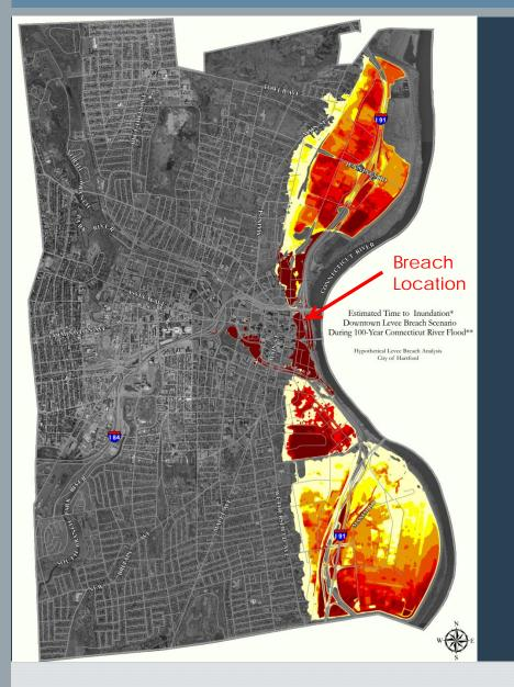
Used computer tools (ArcGIS & HEC-GeoRAS) to simulate a levee breach during a FEMA 100-year flood in each of four neighborhoods and developed maps showing possible timing and extents of flooding
