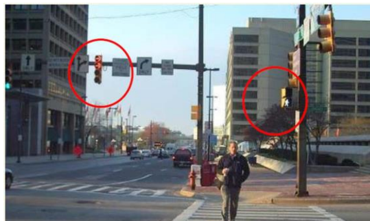
Figure 12 Leading Pedestrian Interval: walk sign lit while vehicle signals are all red, allows pedestrian time to become established in crosswalk before parallel traffic receives a green signal.
