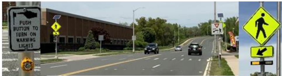
Figure 20 RRFB activation button, street markings, and pedestrian sign with flashers
